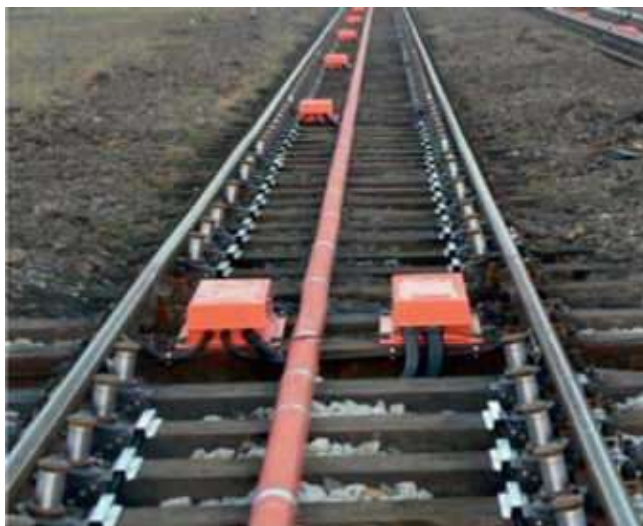
Fig. 1. Placement of retarder fungi at the rail head
